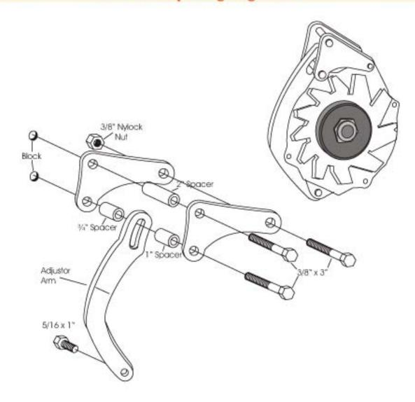
(We use a belt length of  $42\frac{1}{2}$  to  $43\frac{1}{2}$ " with this mount on installations in our shop. However; this can vary with the diameter of your pulleys.)
